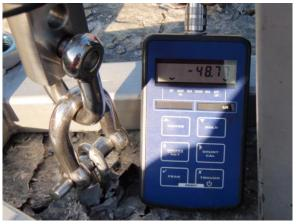
unwound and elongated under loads approaching 50kN. (5<sup>th</sup> anchor from right picture below). The deformation loads were similar to the previous test. The ultimate failure load i.e. the peak load at which the anchor started to egress from the resin or the load required to extract the anchor from the resin, or substrate failure, whichever was higher, was within the range 32 - 63kN with a mean of 44.91kN.
