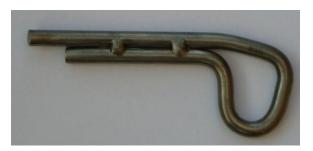
anchor Batch 2". As will be observed later in the report, four out of a sample of sixty four Batch 2 Peco anchors suffered catastrophic metallurgical failure below the 25kN threshold.
